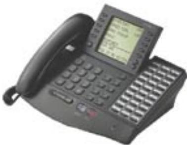
NEC's legendary reliability and quality standards are evident in the DS1000/2000 innovative 32-bit architecture. This new concept **NEC** features Digital Signal Processor (DSP) Technology, on-board flash memory, and field software upgradeability. The compact DS1000 starts with 3 lines, 8 stations, and 4 analog ports. It expands to 6 lines, 16 stations, and 8 analog ports just by plugging in a single expansion board.
